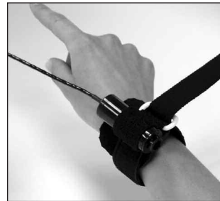
3. Feeding strap through ring, adjust and tighten securing strap to Velcro® hook.
